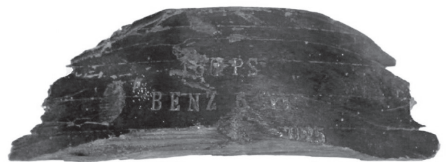
▼ Below: A piece of the LVG.'s propeller marked "150 P.S. Benz 6 Cyl 025." (Xavier Aiolfi)
