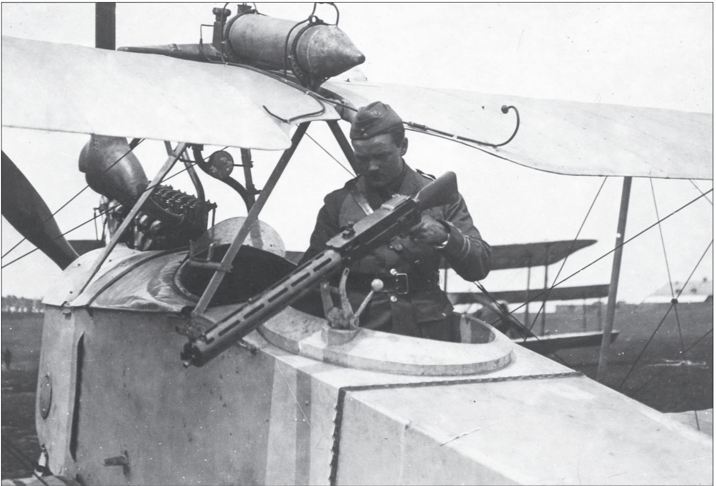
▲ Above: An RFC officer inspects the observer's gun on an LVG C.II captured by the British. This photo was taken at the British airfield at Gouy-Saint André on 28 May 1916. This aircraft is thought to be C.II 2234/15, which was eventually taken to England and exhibited in the Lord Mayor's show in London. The gravity-fed reserve tank is seen on the top wing with its aerodynamic design. ( Bibliothèque de documentation internationale contemporaine )
