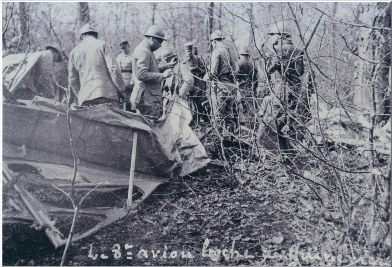
▲ Above: The fuselage broken into two pieces- the rear third of the aircraft lies upside down. ( Bernard Klaeylé )
