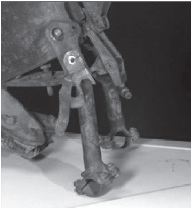
▲ Above: An I.M.G. 08 mounting to an Albatros C.I. Note how the brackets on the C.I. are not connected to one another but are separate pieces. (Peter Grosz)
